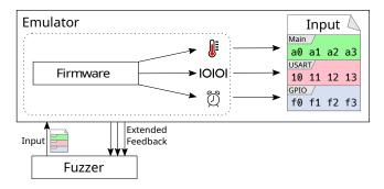
Figure 4: High-level overview of HOEDUR's design. The emulator executes the target firmware in an ISA emulator (dotted). Hardware accesses by the firmware are answered by reading from the data stream that is dedicated to the accessed device. The input file is provided by the fuzzer component. In return, the emulator provides extended feedback to the fuzzer. This feedback is collected during the execution by the emulator.
